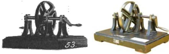
(b) A double-roller slot coupling
