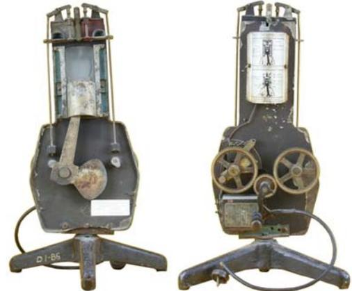
(b) A model with bulb and transformer: front (left) and back (right) views
